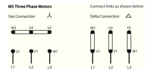
1ph motors are wired differently to 3ph motors and rotation is changed by different positions of the linking bars and supply cables. The wiring for different rotations is as below:
