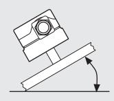
When installed in other positions, the pressure switch switches at pressure deviating from the set reference value by max.  $\pm 0.2$  in. W.C. (0.5 mbar).
