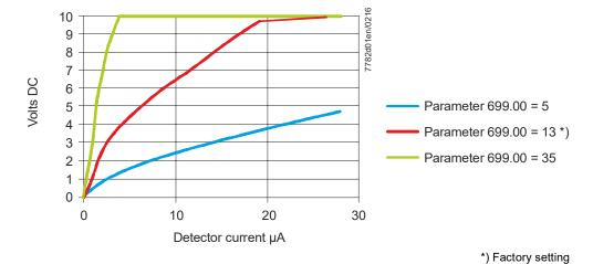
LFS1.2 terminal 7 voltage output for flame supervision with QRA2 / QRA2M / QRA4 / QRA4M / QRA10 / QRA10M
