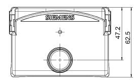
LFS1 with lockout reset button extension AGK20
