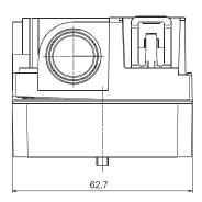
When replacing LAE10 and LFE10 with LFS1, adapter KF8896 ensures that the height can be adjusted mechanically and that the terminals are assigned correctly.
