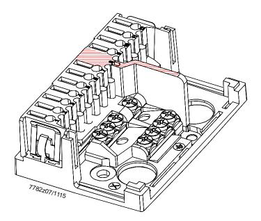
The separating plate must only be plugged into terminal 8
