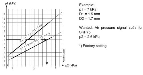
Air is continuously vented to the atmosphere via the damper (D2). The pressure of the following medium will be reduced via throttle «D1». The illustration below shows the correlations.
