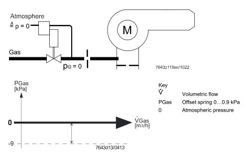
The SKP55 operates with a differential pressure governor and a fixed differential pressure ratio of 1-to-1.
