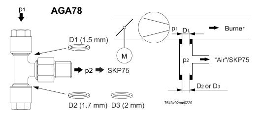
The pressure-reducing T-piece AGA78 is supplied ready for mounting, with D1 = 1.5 mm and D2 = 1.7 mm.
